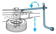
3. Remove the retainer from the spare tire.
